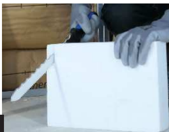
Denture fine pour polystyrène Fine toothting for polystyrene
